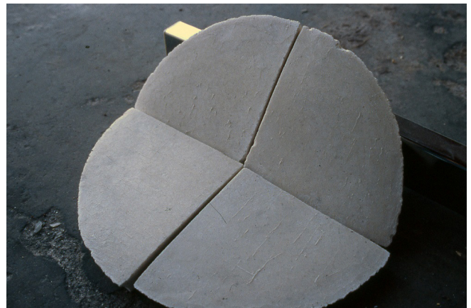
Figure oB-00042b – Nodules on Plaster Surface
