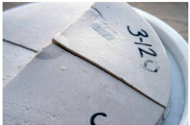
Figure oB-00042c – Absence of Nodules on Molded “Backside” of Plaster Surface
